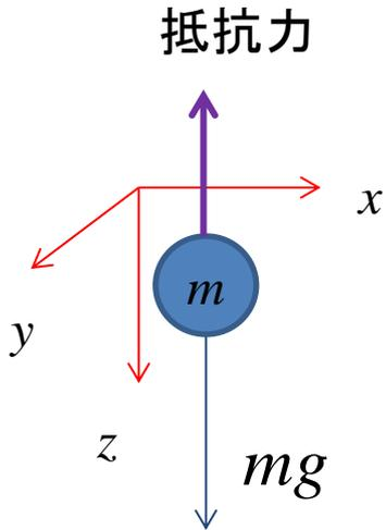
$$-\gamma/m \times (v_z - mg/\gamma) = dv_z/dt$$
